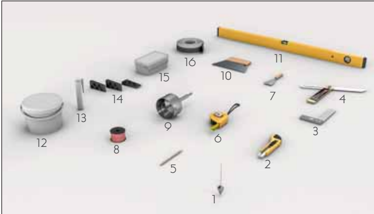
● Optional tools & accessories: 1 Plumb bob, 2 Cutter knife, 3 Set square, 4 Bevel rule, 5 Pencil, 6 Measuring tape, 7 Scraper, 8 Chalkline, 9 Hole saw, 10 Adhesive spreader, 11 Spirit level, 12 Adhesive, 13 Silicone cartridge, 14 Spacer wedges, 15 Sealing coat, 16 Sealing tape.
